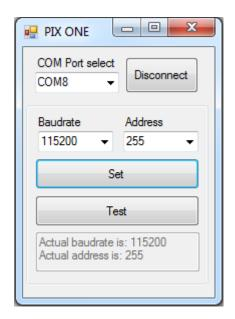
'Set' button is used to send data from 'Baud rate' and 'Address' fields.
